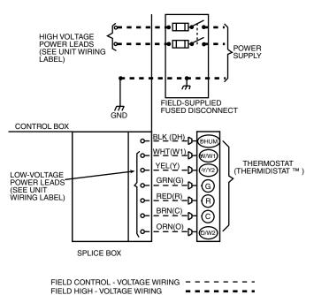
Fig. 3—48JZ High- and Control-Voltage Connections
